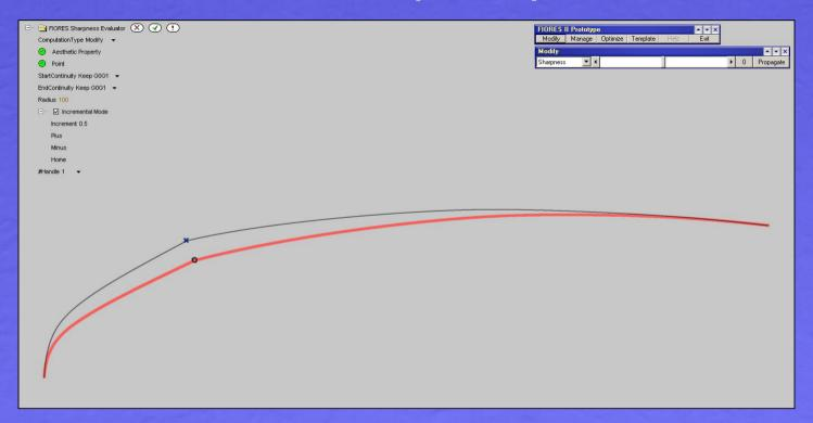
An edge/vertex is perceived *soft* or *sharp* depending on angles between the normal vectors to the surfaces/curves around it. *Crisp* is a qualitative characterisation for *sharp* edges and vertices.
