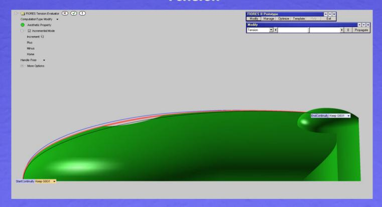
It is (up to some extent) a physical analogy with applying tension to a steel spline
