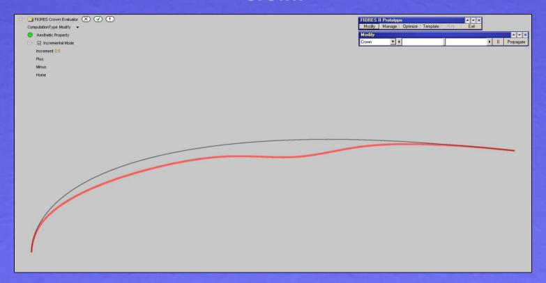
To crown a curve means to lift or raise a (part of) curve while keeping boundary continuity
