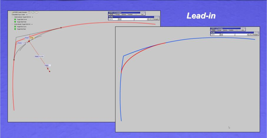
A *lead-in* is the transition of the main curves or surfaces to a *radius*
