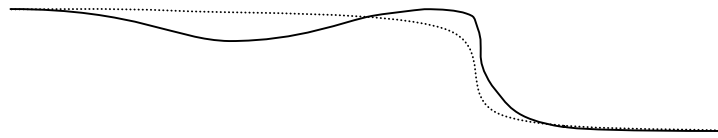
Figure 3. Applying a negative lead in to make a corner look more crisp
