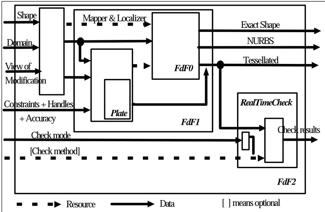
Fig.7: Component software architecture
