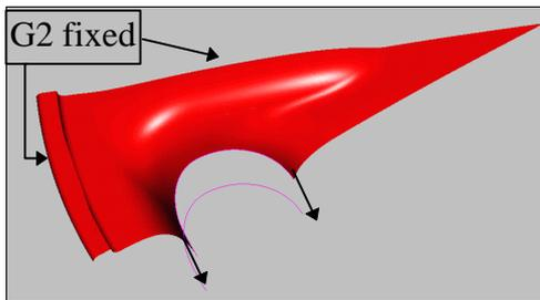
Fig.8: Rim part before deformation
