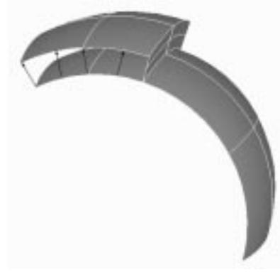
**Figure 9:** Representation of an offset-up surface
